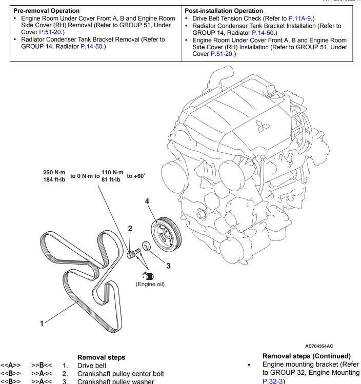
>>A<< 3. Crankshaft pulley washer
