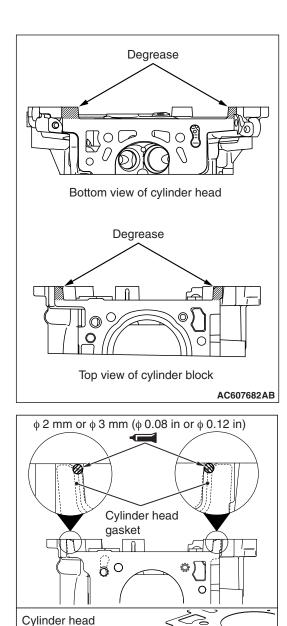
2. Apply the sealant to the top surface of cylinder block as shown in the figure.
