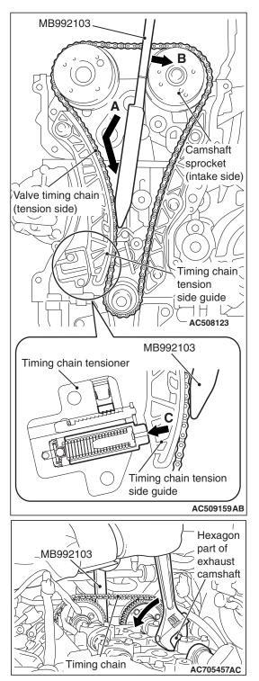
2. With the timing chain tensioner unlocked, insert special tool MB992103 inside the timing chain case assembly along the tension side of the timing chain until the insertion guide line aligns with the upper surface of the timing chain case assembly (Figure A.)
