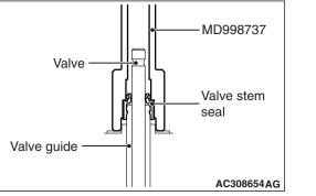
2. Use special tool MD998737 to press-fit a new valve stem seal in the valve guide using the valve stem area as a guide.
