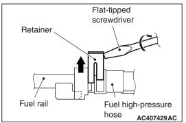
(1) Insert a flat-tipped screwdriver [6 mm (0.24 inch) wide and 1 mm (0.04inch) thick] into the retainer of the fuel high-pressure hose connector.
