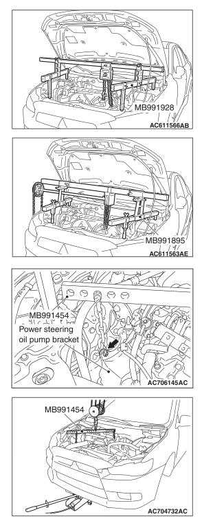
2. Remove special tool MB991928 or MB991895 which was installed for supporting the engine assembly when the transaxle assembly was removed (Refer to GROUP 22C, Transaxle Assembly P.22C-497.)
