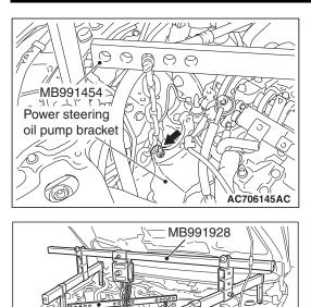
(3) Mount special tool MB991454 to the power steering oil pump bracket and engine hanger, and set it to special tool MB991928 to support the engine and transaxle assembly.
