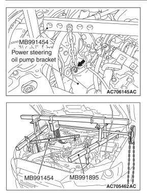
(2) Mount special tool MB991454 to the power steering oil pump bracket and engine hanger, and set it to special tool MB991895 to support the engine and transaxle assembly.
