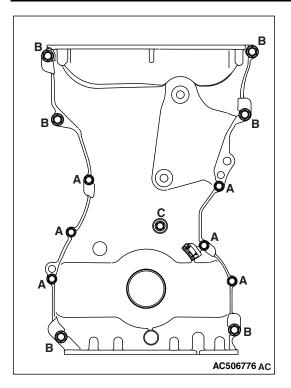
6. Insert the bolts to the timing chain case assembly as shown, and tighten them to the specified torque.
