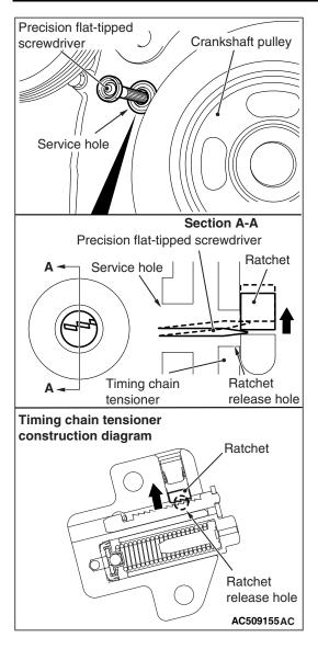
2. In the same manner as removal, insert the precision flat-tipped screwdriver through the service hole of the timing chain case assembly, press up the ratchet of timing chain tensioner to unlock, and hold the unlocked timing chain tensioner.
