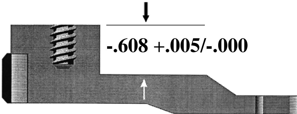
It is important to maintain the proper flywheel step specification. Failure to maintain the proper step specification may result in poor clutch performance, slippage, and/or improper release.
